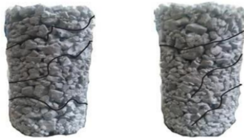
Figure 8. Crack Pattern of 3 days porous concrete with Slag Nickel and Broken Stone
